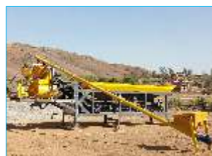
Mobile Batching Plant
