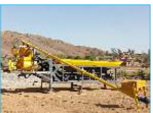
Mobile Batching Plant
