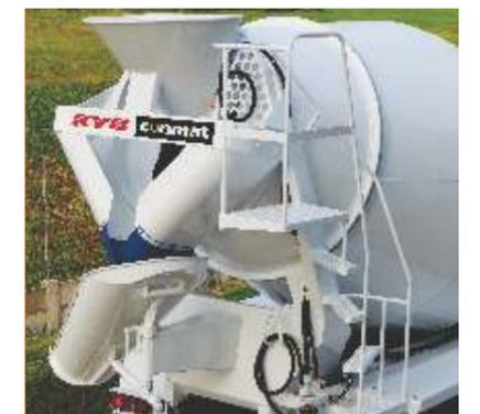
Staircase to inspection platform is designed for operator comfort without compromising safety
